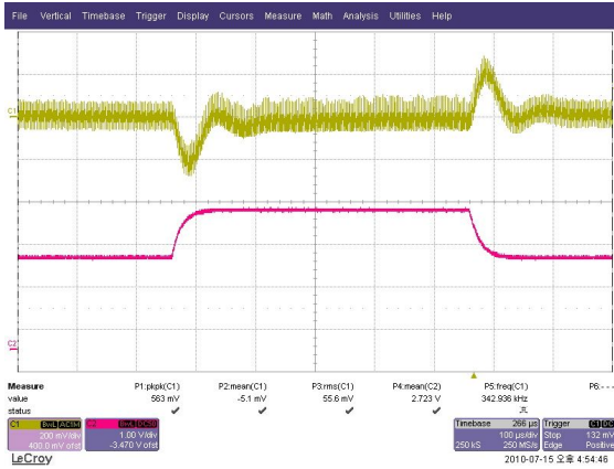
[Fig.3] Load step: 50%-75%-50% of I_o , di/dt=0.1A/\mu s (CH1: 200mV, CH2: 1A/div, 100us/div)
